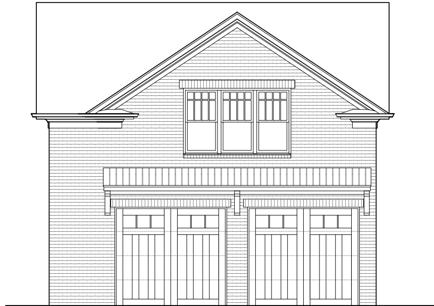
1 GARAGE FRONT ELEVATION 1/8" = 1'-0"
